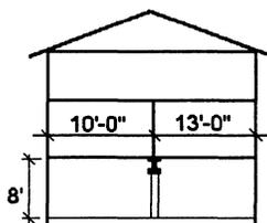
**Solution:** One continuous beam with two columns equally spaced is chosen. The top flange of the beam is to be braced at each joist (a positive connection is necessary between each joist and the beam). Provide a minimum of 1¾ inches of bearing at the beam ends and 3½ inches of bearing at each column.
