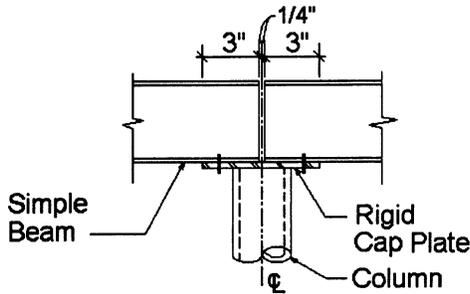
Each beam end is ¼ inch from the column centerline and the bearing length is 3 inches. Therefore the eccentricity for each beam reaction is ¼ + 3/2 = 1¾ inches (dimension from the centerline of bearing to the centerline of the column). Under full load the eccentric loads counteract each other and do not induce any moment into the column. The maximum unbalanced load condition occurs when all the live load is on one beam. Therefore this case has to be checked.
